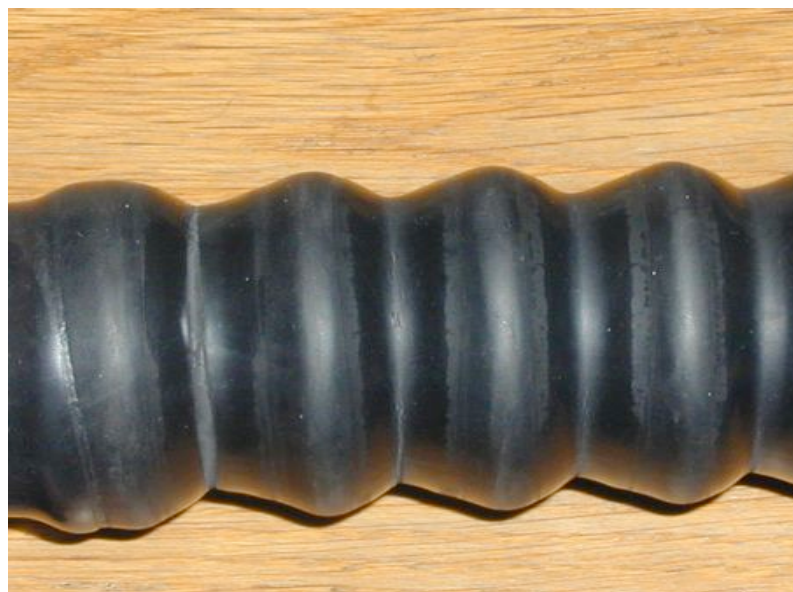
Fig 1:: Hose with jubilee clip, after tensioning the clip until the grub screw failed, then tensioning the hose until the hose failed. Hose failure point is at the same point observed in the tests reported in the FMECA Vol 4
