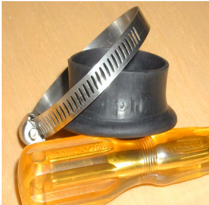
Fig 1:: Hose with jubilee clip, after tensioning the clip until the grub screw failed, then tensioning the hose until the hose failed. Hose failure point is at the same point observed in the tests reported in the FMECA Vol 4
