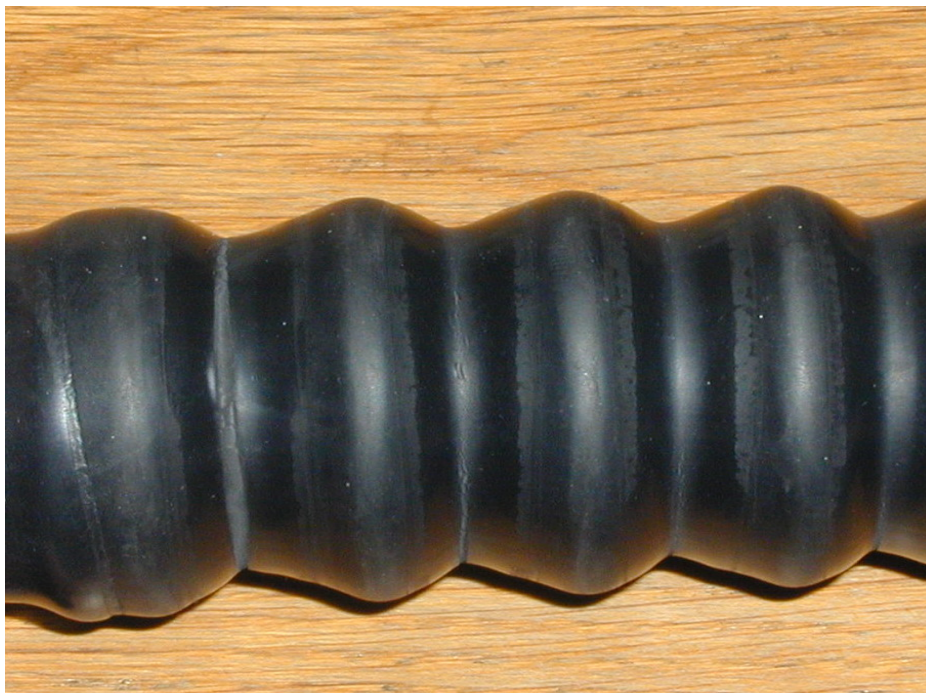
Fig 2:: Hose under tension showing cracks caused by forming tool during manufacture, from which failures extend around the hose.
