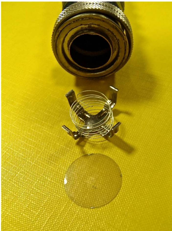
Figure 2-1: IDA-71 inhale valve. The valve has an opening pressure of around 1mbar, and provides an extremely low work of breathing. It cannot suffer from turbulent bypass: the fault mode considered in this report.
