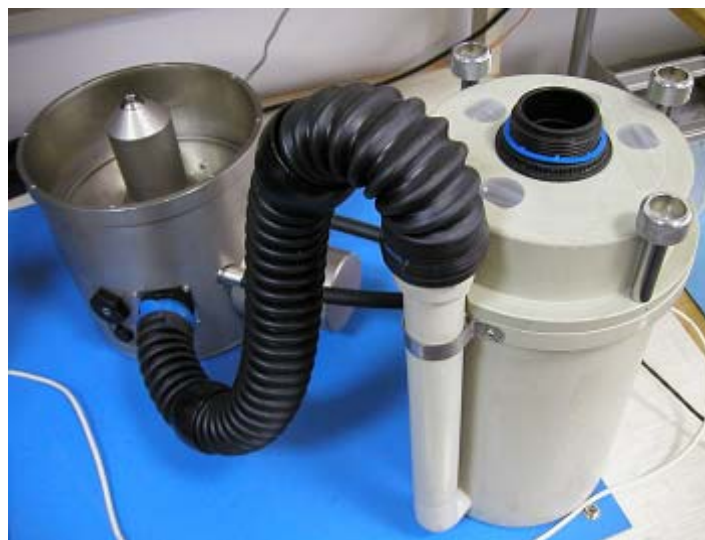
Fig 4-12. Position of scrubber canister. Note the electronics was removed and the ports blocked with tape, as the purpose was to measure the scrubber canister characteristics, not that of the electronics.
