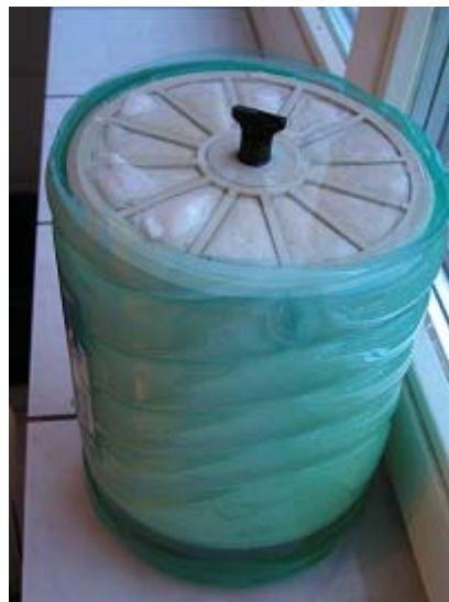
Fig 4-18. Cartridge in water. After two hours, it was removed and transferred straight into the scrubber housing.
