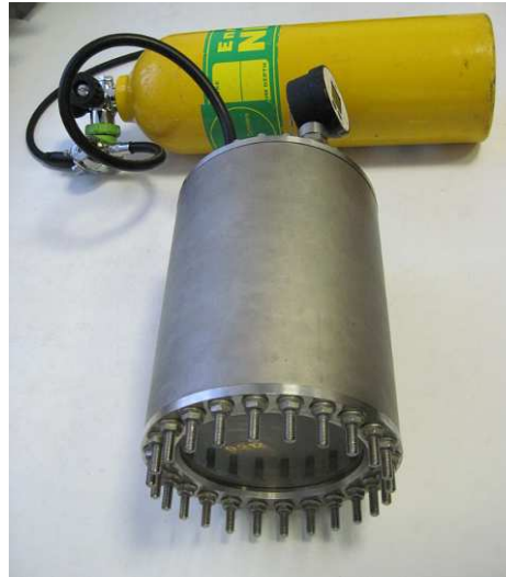
Figure 10-1. Variable pressure test fixture for the PPO2 Pod
