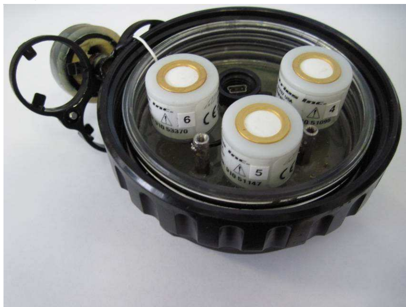
Figure 27: O 2 cell bath N2 in the pod, cell retainer removed to provide unobstructed view of the oxygen cells.
