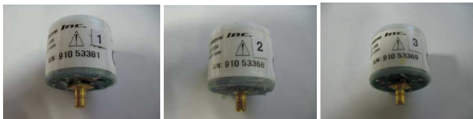
Figure 1: Oxygen sensor test batch N1, manufactured in October 2009, tested in January 2011 to a Deep Life Procurement Specification [1]. When new, these have an output of nominally 5mV in air. These cells are not temperature compensated internally: they are used with external digital temperature compensation.
