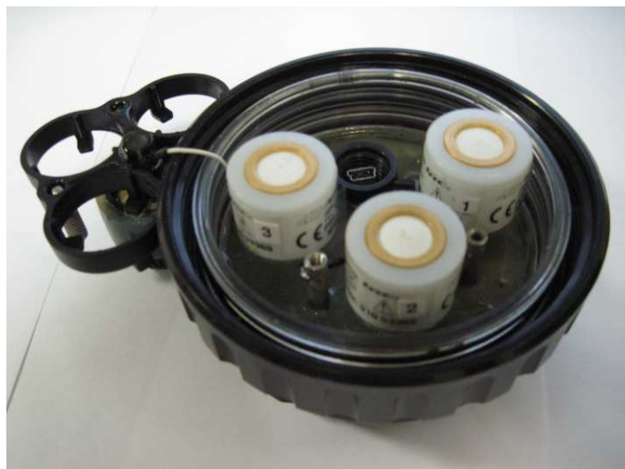
Figure 3: Oxygen Monitor with O2 cells prior to test (cell holder disconnected and seen on top left of image to provide a clear view of the cells).
